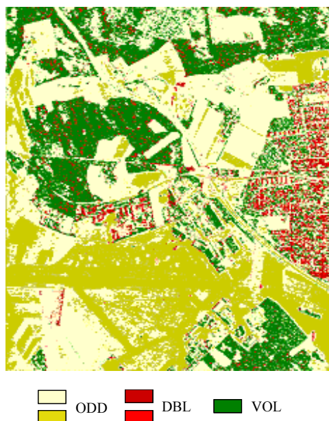
Fig. 13: Selection of significant mechanisms and identification to canonical scattering mechanisms (ODD: Single Bounce Scattering, DBL: Double Bounce Scattering, VOL: Volume Diffusion)
